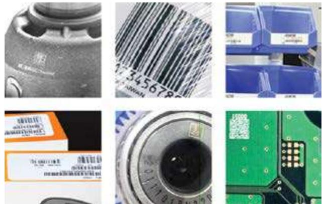
Figure 6. Code substrates affect reflectance differently and influence lighting angles.
