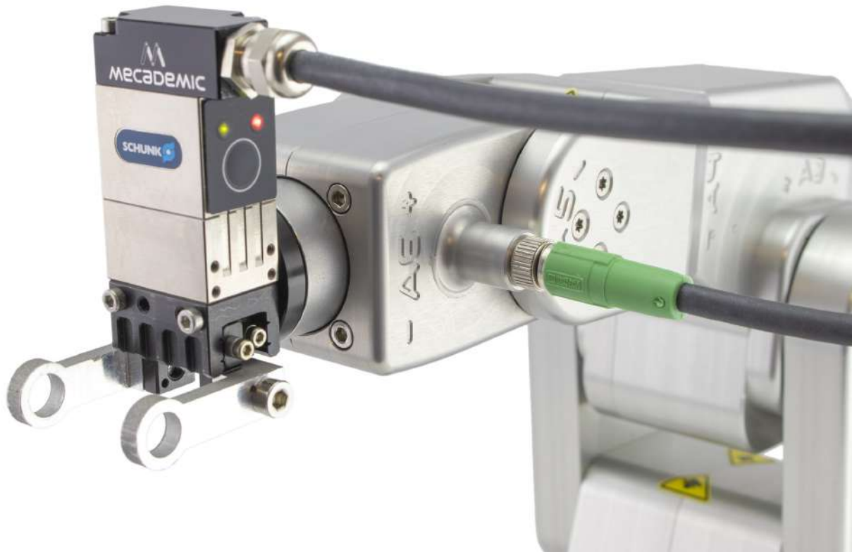
Figure 5: The MEGP 25 completely installed and homed
