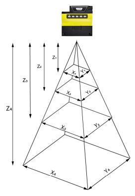
The following table shows the Field of View (FoV) widths of the 6.2 mm lens focused to 190 mm at various distances.
