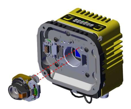
Tighten one of the M2 x 8 mm screws halfway, then tighten the other M2 x 8 mm screw halfway. Incrementally tighten each screw to 0.34 Nm using a torque wrench.
