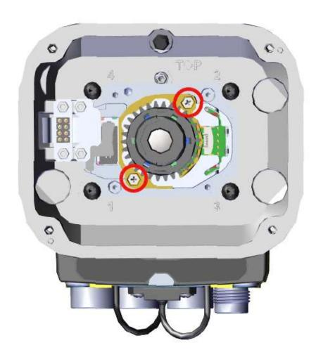
6. Replace the adapter on the sensor.
