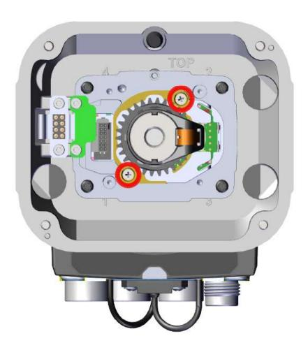
3. Remove the lens from the sensor.
