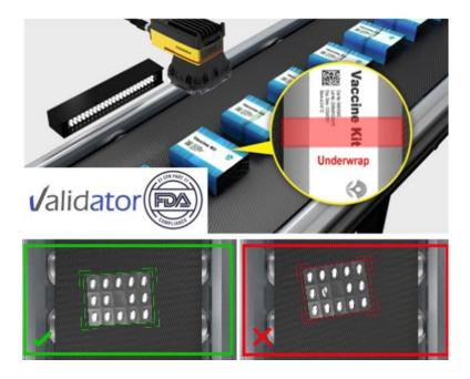
100% inspection of a blister was required to ensure the correct size and colour tablet `or capsule has been dosed into the blister. Any missing tablets, incorrect variant or broken tablets will be rejected in a controlled method.
