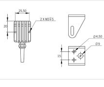
During the set up, the light has to be switched off and unplugged. Please use the fixing holes designed for that purpose (see scheme above). We recommend the using of M3 screws (not supplied) with a tightening torque from 0.5 to 1.5 Nm. We also recommend the use of a threadlocker (not supplied) to avoid any risk of loosening.
