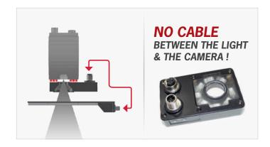
The **Optical Trigger** is an easy solution to connect the MR-RING to your smart camera, **without a wired connection**. Whenever the camera's **embedded light** is on, the Optical Trigger automatically sends a signal to the external light. Using the Optical Trigger, you can get a perfect **synchronization** of the MR-RING with the camera software very easily.
