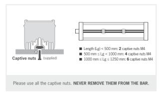
During the set up, the light has to be switched off and unplugged. Please use M4 screws and insert them in the captive nuts located in the back of the light. The light will be better fixed if you spread the attachment points symmetrically along the bar.
