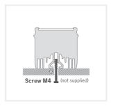
You can also use M4 screws (not supplied) fastened directly into Aluminium profile with a tightening torque from 0.5 to 1.5 Nm. We also recommend the use of a thread-locker (not supplied) to avoid any risk of loosening.
