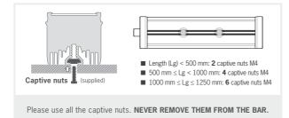
During the set up, the light has to be switched off and unplugged. Please use M4 screws and insert them in the captive nuts located in the back of the light. The light will be better fixed if you spread the attachment points symmetrically along the bar.
