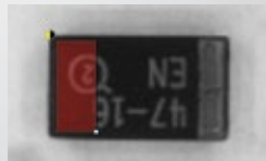
Capacitor Oriented Backwards
