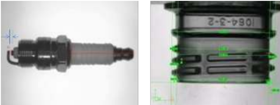
Figure 7. Gauging applications can measure part tolerances to within 0.0254 millimeters.
