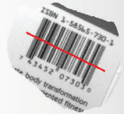
Figure 5a. Barcode at 1.2 PPM, with projection line
