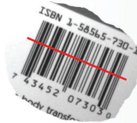
Figure 4a. Barcode at 1.5 PPM, with projection line
