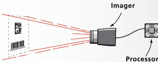
**Figure 2.** Conventional image-based reader technology. Note the horizontal width and a vertical height, which defines the scene the camera can see. The camera field of view gets wider as you move away from the lens but each pixel covers more area. At some distance the reader can no longer distinguish the cells or modules of a code.
