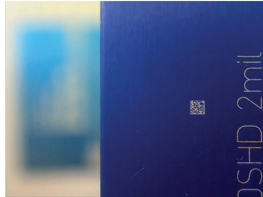
The liquid lens adjusts for a small close up Data Matrix code, above, and below can focus on barcodes at a distance.
